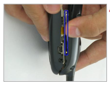
▲ Do not try to pull the two pieces apart. You may tear the antenna cable. Instead, fold the two pieces open to avoid stress on the cable.
