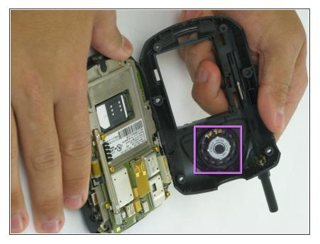
Separating the two halves allows you to access the speaker. Which is located in the front half of the case.
