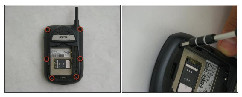
• Use a T6 Torx screwdriver to remove the six screws located on the rear of the phone.
