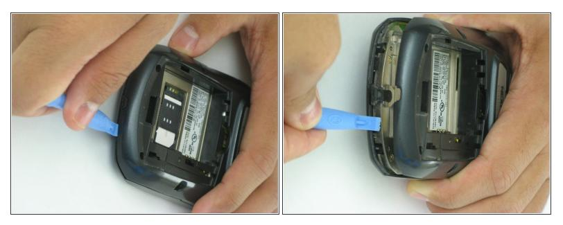
Use a pick or plastic iPod opening tool to push the clips, that are holding the rear casing. Apply a firm pressure at a forty-five degree angle to dislodge the clips.
