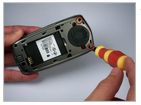
Remove top two screws with T6 Torx screw driver, from the back of phone.
