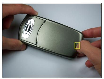
Press your thumb against the battery latch. While pressing on latch, slide off battery cover towards the bottom of the phone.
