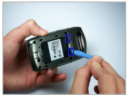
Remove speaker phone cover by unsecuring the two latches on the edge close to top of the phone with the plastic opening tool.
