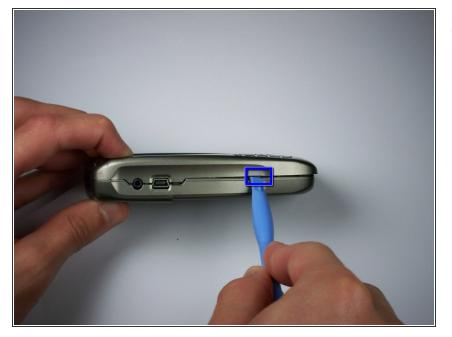
Turn the phone sideways and unlatch the hinge on one side of the phone by pushing inwards and twisting to the side with the plastic opening tool.
