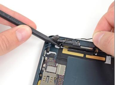
Use the tip of a spudger to remove the small piece of tape securing the antenna cable in the bottom right corner of the iPad.
