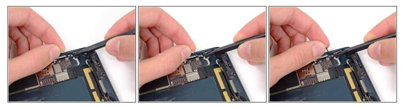
Use the tip of a spudger to pry the small metal retaining clip off the left antenna cable, then deroute the cable from the clip.
