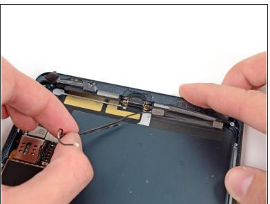
Pull the antenna cable from the slot behind the Lightning connector.
