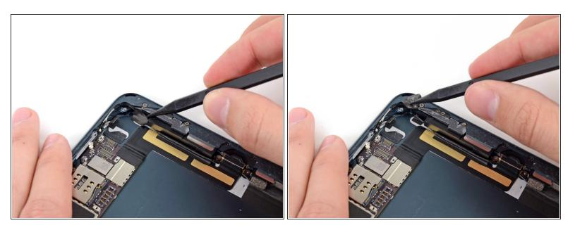
With the tip of a spudger, peel up the larger piece of tape covering both antenna cables near the bottom of the rear case.
