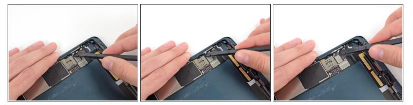
Use the flat end of a spudger to disconnect the two bottom antenna cable connectors from their sockets on the logic board.
