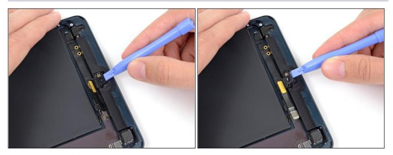
• Use a plastic opening tool to gently pry the front-facing camera forward, separating it from the adhesive securing to the rear case.
