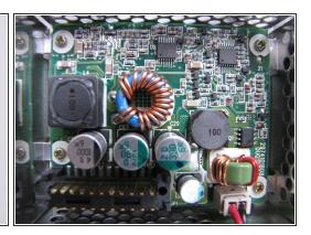
• If you lift the mainboard up, you'll see a metal plate, probably for EMI-protection. Remove the two screws holding it and you have access to the internal power supply.
