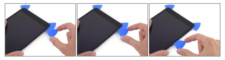
Insert a new opening pick and slide it to the middle of the right edge of the iPad, releasing the adhesive as you go.
