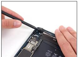
With the tip of a spudger, peel up the larger piece of tape covering both antenna cables near the bottom of the rear case.
