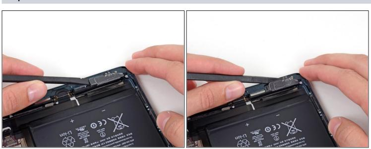
• Use the flat end of a spudger to loosen the foam adhesive securing the Wi-Fi/Bluetooth antenna to the left speaker.
