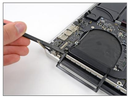
Use the flat end of a spudger to carefully pry off the rubber screw cap on the raised screw head near to the MagSafe 2 connector.
