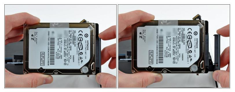
Disconnect the hard drive by pulling the hard drive cable connector away from its socket on the hard drive.
