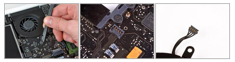
• Use a spudger to pry the fan connector straight up and out of its socket on the logic board.
