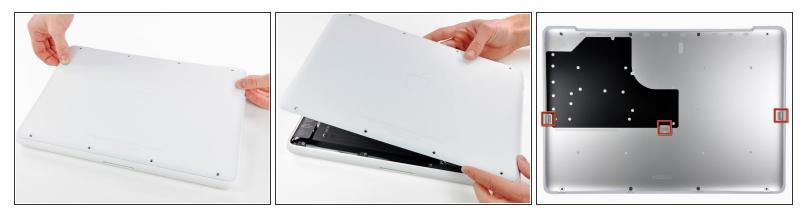
A The lower case is constructed of rubber-coated aluminum. Do not excessively bend the aluminum during removal, as any permanent deformation will cause tolerance issues after reassembly.
