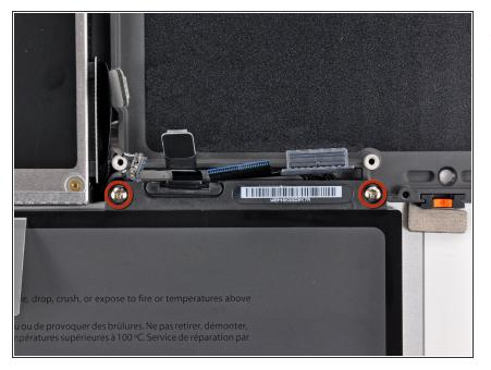
Remove two 5 mm Tri-Wing screws securing the battery to the upper case near the battery connector.
