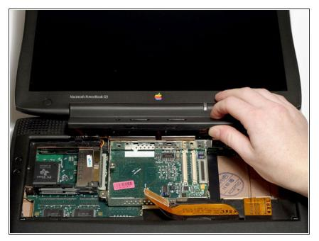
• Lift the clutch cover off by rotating it up and then toward you.
