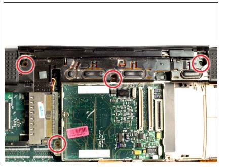
• Remove the four T8 Torx screws from the upper case.
