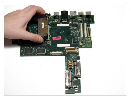
Clasp the PC card cage between your thumb and index finger and lift it directly upward.
