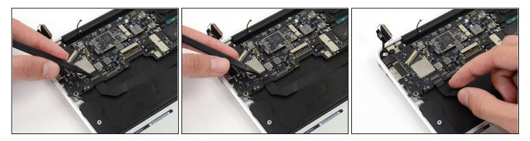
• Use the tip of a spudger or your fingernail to flip up the retaining flap on the trackpad ribbon cable ZIF socket.
