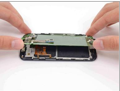
Gently lift the motherboard out of the phone, rotating it from the SIM slot edge of the phone.
