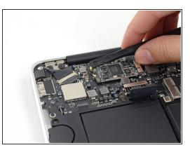
Use the flat end of a spudger to pry both antenna connectors up from their sockets on the AirPort/Bluetooth card, and move them out of the way.
