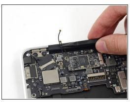
Use the tip of a spudger to de-route the antenna cables from their notches in the logic board.
