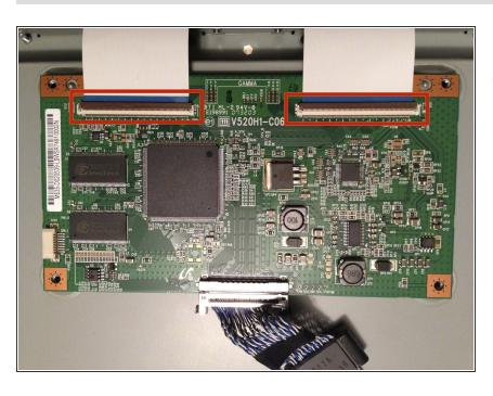
Disconnect the two ribbon cables at the top by flipping up the retaining flaps and sliding the ribbons straight up towards the top of the TV.
