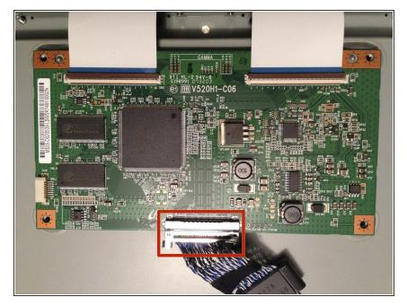
Disconnect the bottom ribbon cable by depressing the two buttons on either side of the connector and sliding down towards the bottom of the TV.
