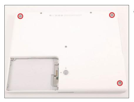
Remove the three newly-revealed Phillips screws.
