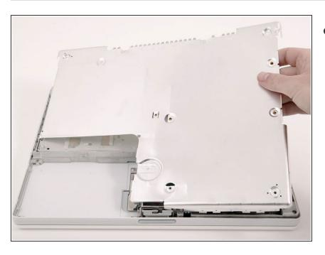
Lift the bottom shield off.
