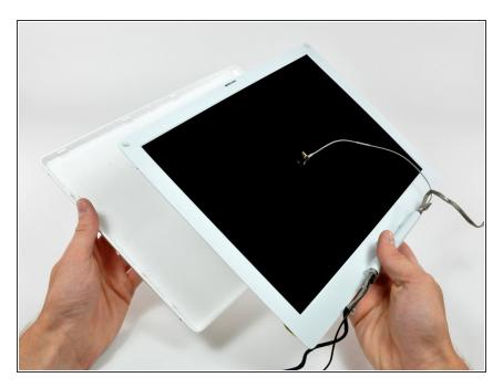
Lift the rear bezel off the display.
