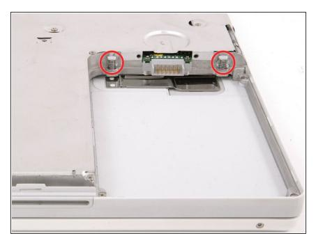
Remove the small greasy springs with white plastic caps from either side of the battery contacts.
