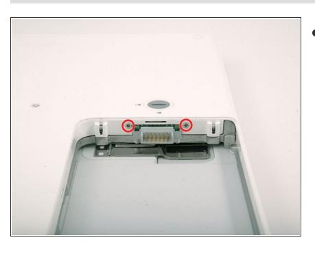
Remove the two Phillips screws on either side of the battery contacts.
