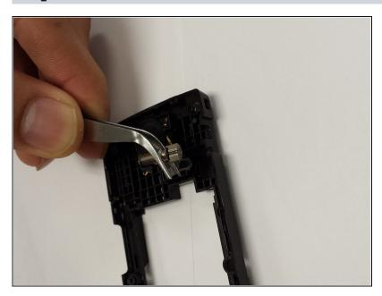
The antenna is located on the opposite side of the black plastic cover. Use the tweezers to remove the antenna.
