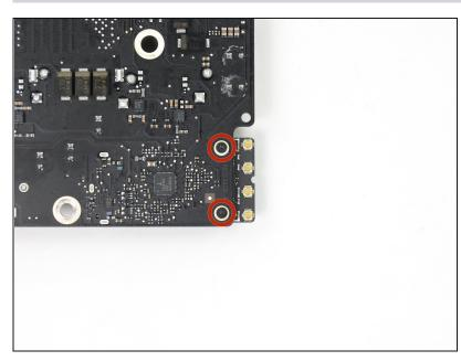
Remove the two 3.2 mm T5 screws securing the AirPort/Bluetooth card to the logic board.
