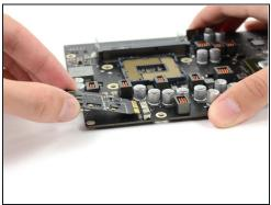
• Lift the end of the AirPort/Bluetooth card slightly, and pull it straight out of its socket on the logic board.
