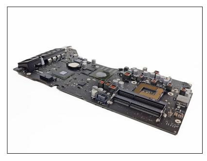
During reassembly of the logic board, pay attention to the position of the I/O connectors. When the board is back in the case, insert a USB or Thunderbolt cable into one of the connectors to align it perfectly.
