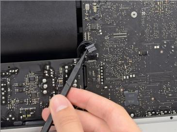
• Gently push upward on each side of the power supply control cable connector with the tip of a spudger to gently "walk" it out of its socket.
