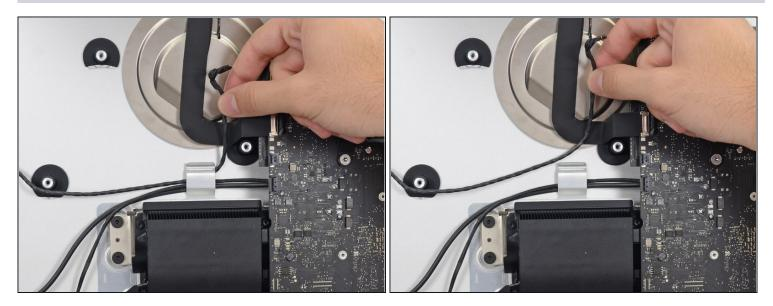
• De-route the left speaker cable by pulling it straight up out of the retaining clip in the back of the rear enclosure.
