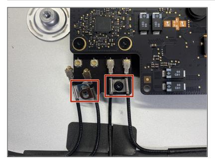
If brackets secure the four antenna cables, remove the two T5 Torx screws from the brackets.
