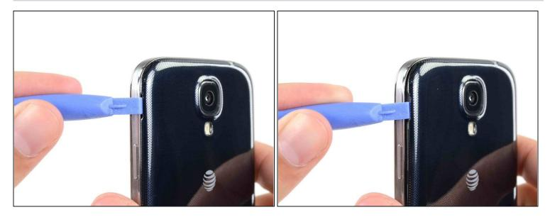
• Pry with a plastic opening tool, or your fingernail, in the divot to the left of the rearfacing camera, near the power button.
