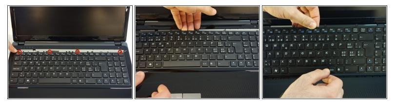
• Use a Phillips # 1 screwdriver to remove the four screws securing the keyboard in the upper part.
