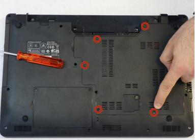
Using a Philips #1 screwdriver, unscrew the 5 screws securing the cover.
