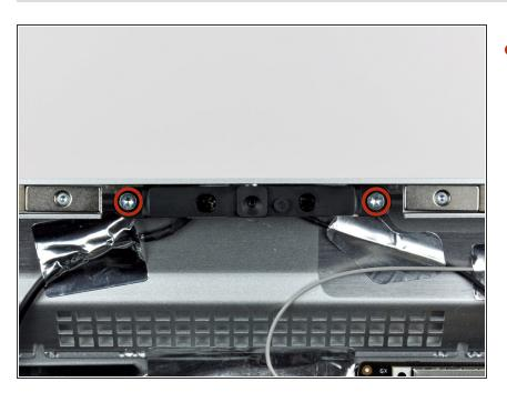
Remove the two T10 Torx screws securing the camera board to the outer case.
