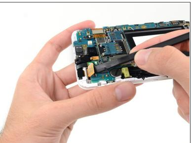
Use the flat end of a spudger to carefully disconnect the display cable connector.
