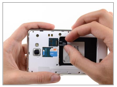
• Remove the microSD card from its slot in the midframe.
