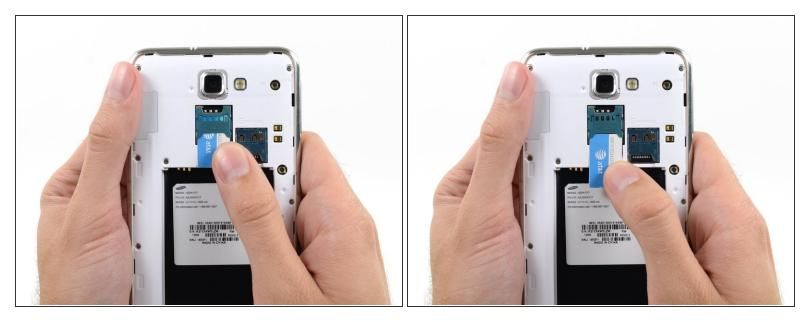
• Slide the SIM card out the rest of the way with your thumb and remove it from the device.
