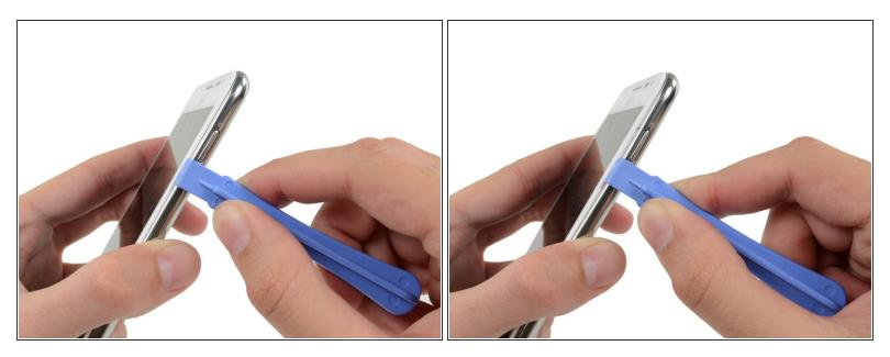
Insert your plastic opening tool to the left of the power button between the midframe and the front panel assembly and pry.
