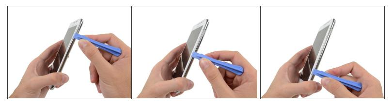
• Slide the plastic opening tool down the seam.
