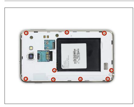
Remove the nine 3.4 mm Phillips #00 screws securing the midframe to the display assembly.
