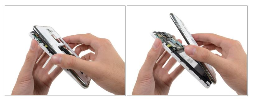
• Remove the midframe from the display assembly.
