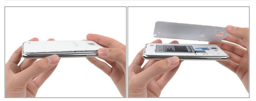
• Lift and remove the rear case from the phone.
