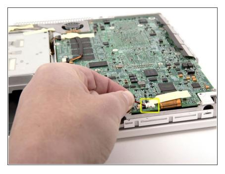
Turn the computer over and disconnect the sleep light from the logic board. To reassemble your device, follow these instructions in reverse order.
