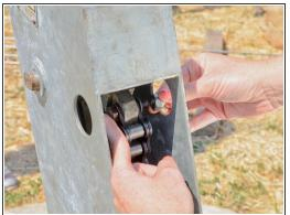
Remove the nut from the chain bolt.
