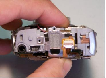
Remove the A/V port cover [no tools are necessary]
