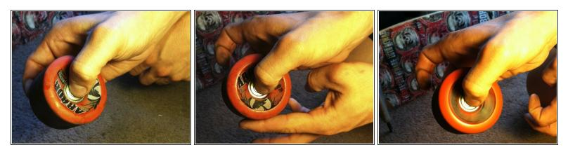
• Spin the wheel to make sure that the bearings are properly aligned and running smoothly.
