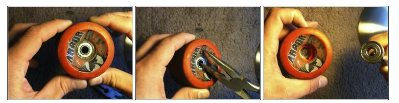
• Use needle nose pliers to remove the bearings from both sides of each wheel.
