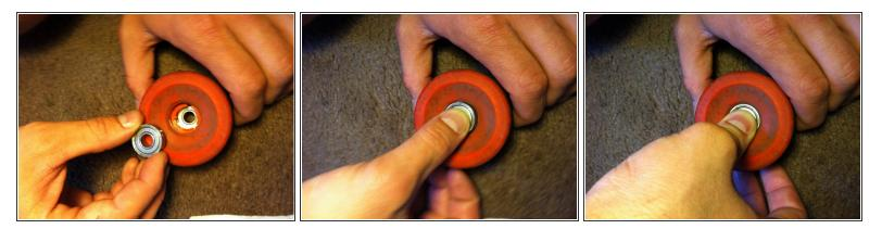
• Push the bearing into the wheel by applying even pressure with your thumb.
