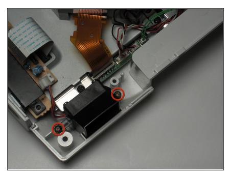
• Remove the two 8.5mm Philips #00 screws from the fan bracket.
