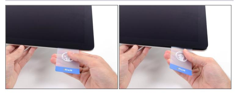
• Gently twist the card, slightly increasing the space between the display and frame.
