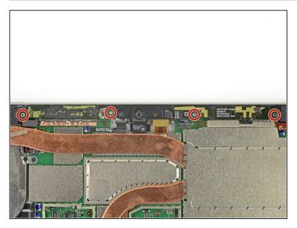
Use a T5 Torx screwdriver to remove the four 4.5 mm screws securing the antenna support bracket.
