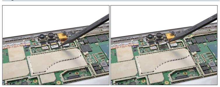
Use the pointed end of your spudger to disconnect the front camera from the motherboard.
