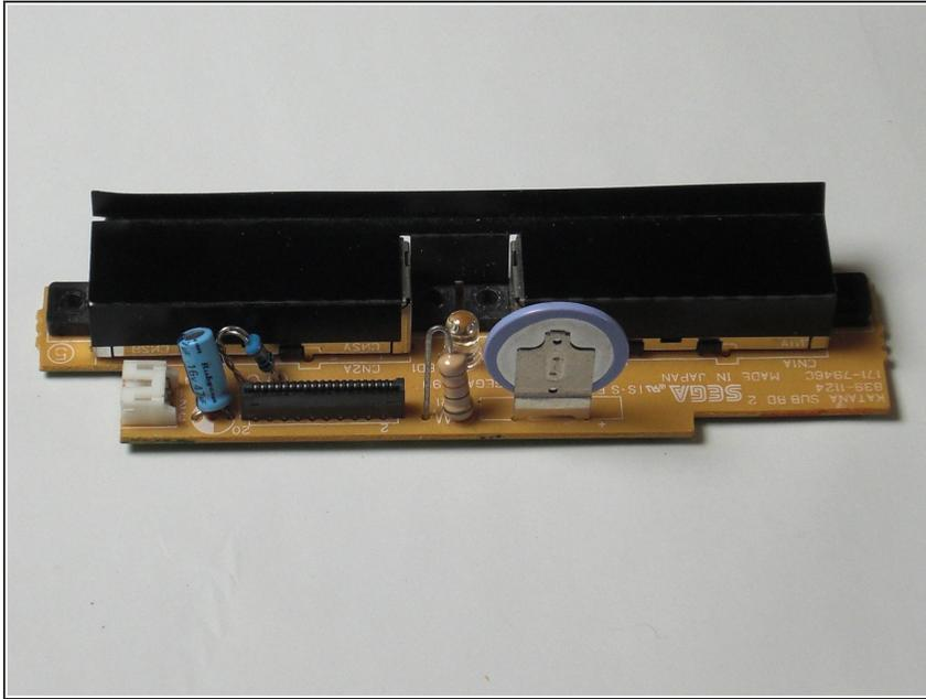
**⚠ Verify that the resistor(s) leads do not touch other components on the topside of the circuit board. Otherwise, a [short circuit](#) may occur when you power on the system.**
