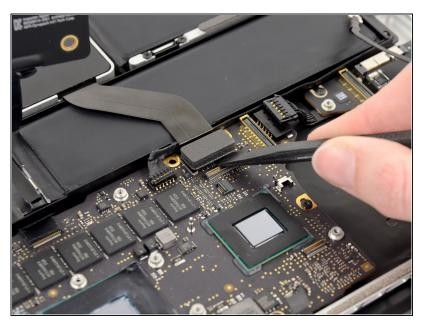
Use the flat end of a spudger to pry the SSD cable connector up off its socket on the logic board.
