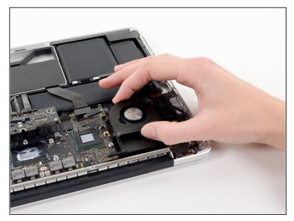
• Lift and remove the right fan out of the upper case.
