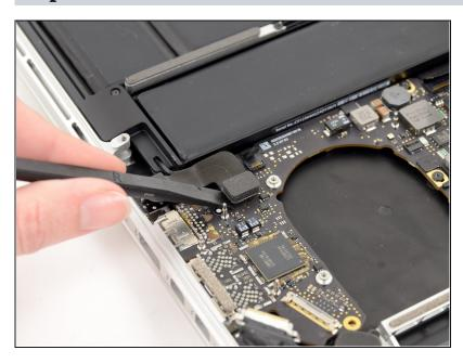
Pry the headphone jack cable connector up off its socket on the logic board.
