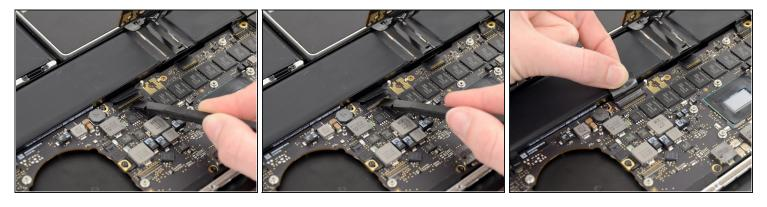
• Use the flat edge of a spudger to flip up the retaining flap on the keyboard ribbon cable ZIF socket.
