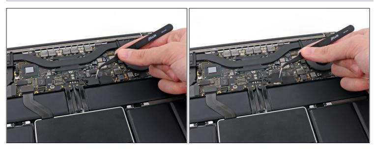
• Use <u>tweezers</u> to remove the small plastic cover located near the bottom right of the battery connector board.
