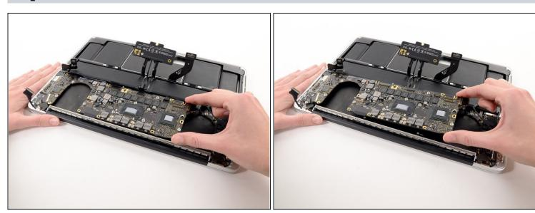
• Carefully grasp the corner of the logic board (opposite of the I/O ports) and lift the logic board out of the upper case.
