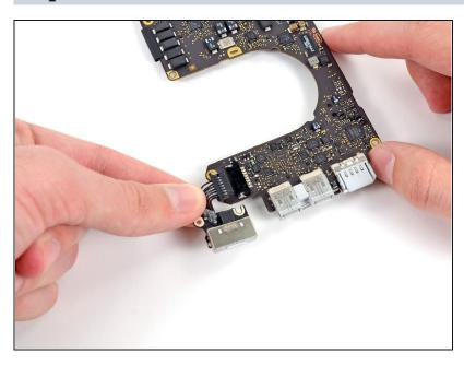
Pull the MagSafe cable connector straight out of its socket on the logic board.
