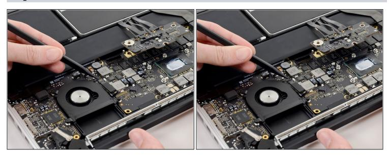
• Use the tip of a spudger to flip up the retaining flap on the left fan ribbon cable ZIF socket.
