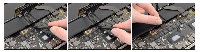
• Repeat the previous procedure to disconnect the Trackpad ribbon cable from its socket on the logic board.
