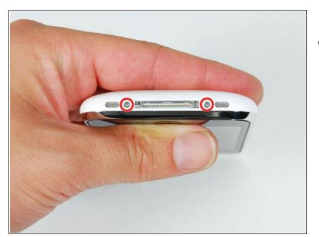
Remove the two Phillips #00 screws from the dock-connector end of the iPhone.
