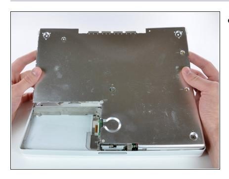
• Lift the bottom shield off.
