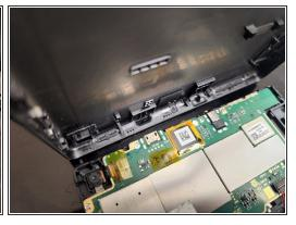
Lift the back cover off, tilting towards the top as if it was a hinge. There are no cables or wires connecting the back, but be careful around the top of the device. All the buttons and connections are on this edge and lifting this edge up could damage them.
