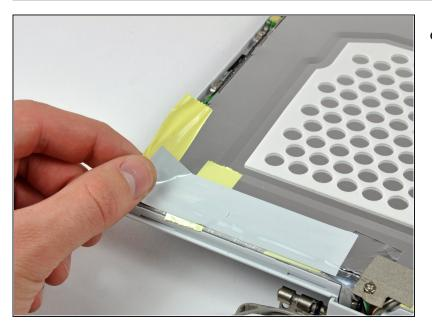
Remove the large piece of tape near the lower right corner of the display.
