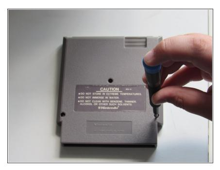
Remove the three screws on the bottom of the cartridge. While most of the time the screws are security screws, sometimes there are Phillips/Flathead screws.
