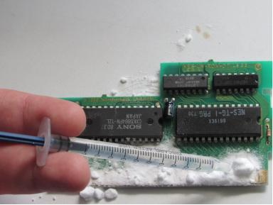
Simply put about 2 tablespoons of baking soda on the cartridge contacts. Then put enough water on the baking soda until it is the consistency of a thick paste.
