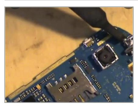
Removing the charging port with the use of a soldering iron or hot air
