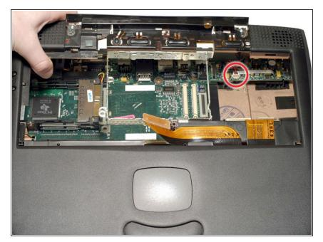
Grasp the upper case near the back left corner and lift up partly so that you can access and disconnect the
