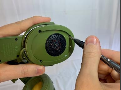
Remove three 12 mm Phillips #1 screws located underneath the left ear cushion of the headphones.
