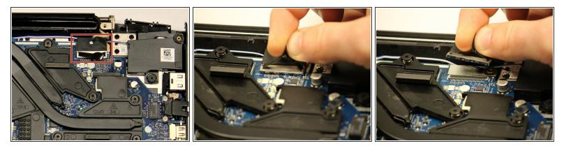
• Grab the black tab on top of the cable and pull up to unplug.
