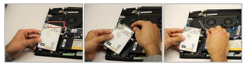
• Finally, unplug the hard drive from the motherboard by pulling to disconnect the highlighted cable.
