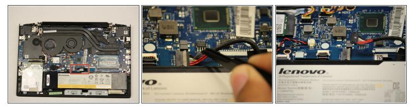
• Disconnect the battery from the motherboard.
