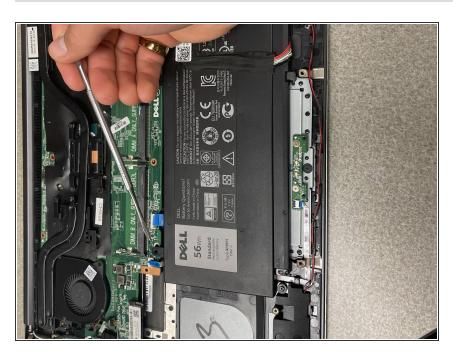
Disconnect the battery ribbon connector.
