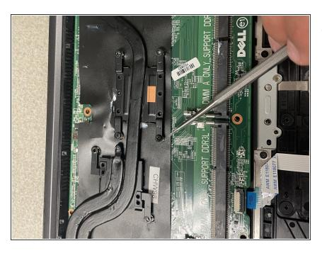
Remove the screws securing the heat sink.
