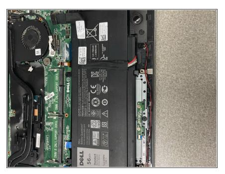
Remove the screws holding the battery.
