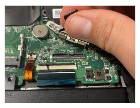
Disconnect the display screen ribbon connector.
