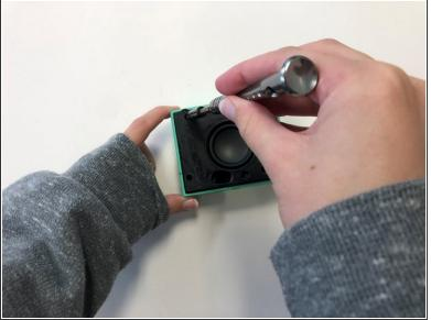
Once the front cover is removed, use a T6 screwdriver head to remove the four 9 mm screws on the black cover.
