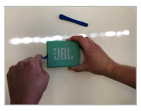
Once you have scraped off all of the glue, use the opening tool to pry up the front cover.
