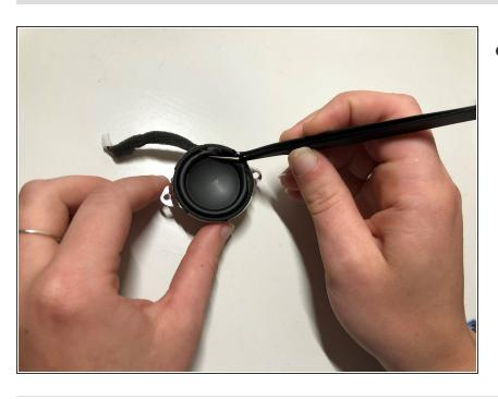
Once the woofer is removed, use sharp tweezers to carefully remove the foam surround from the woofer.
