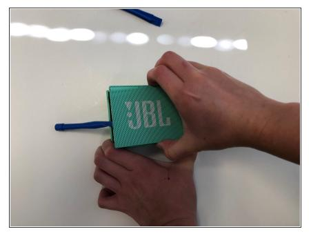
• Carefully remove the loose plastic cover from the speaker.
