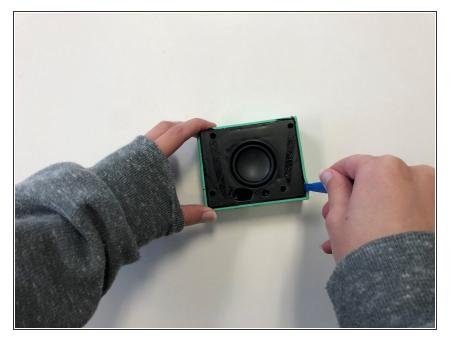
After removing the screws, use the plastic opening tool to carefully pry around the edges of the black cover to loosen and lift the cover off of the device.
