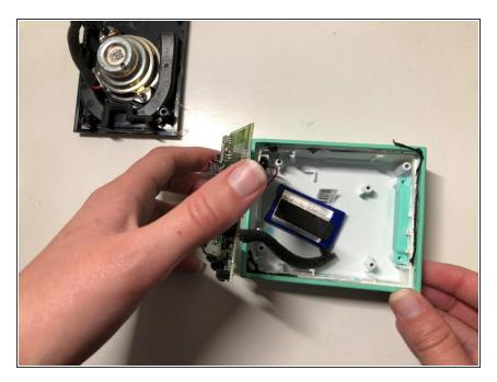
• Lift the motherboard using the plastic opening tool and stick it through the hole in the middle of the board.
