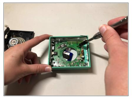
• Use the T6 screwdriver to remove the 9 mm screw that secures the motherboard in place.
