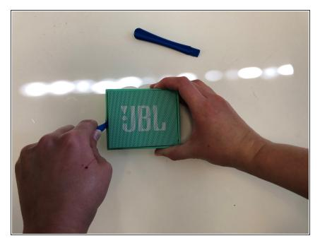
• Once you have scraped off all of the glue, use the opening tool to pry up the front cover.
