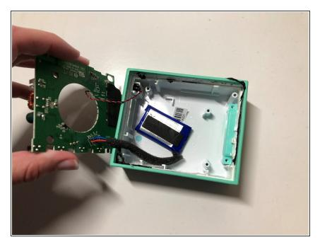
• Carefully lift the motherboard, sliding the charging port side out of the frame of the speaker as you go.
