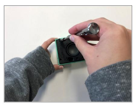
Once the front cover is removed, use a T6 screwdriver to remove the four 9 mm screws on the black cover.
