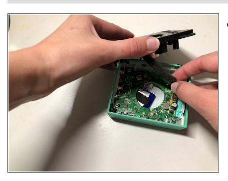
Carefully unplug the woofer wires from the motherboard
