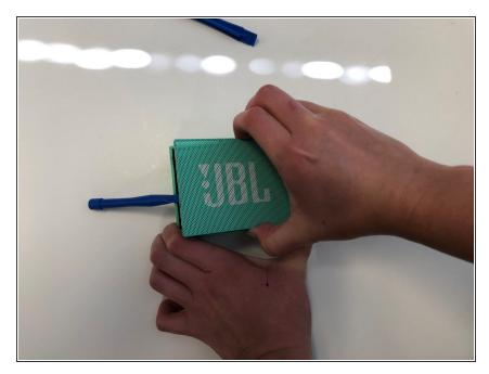
Use an opening tool to scrape around the outside of the front cover to remove the glue attaching it to the surrounding rubber layer.
