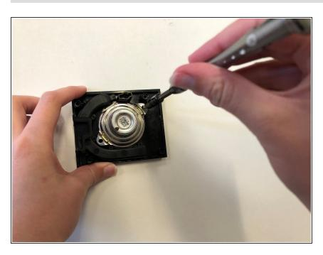
Once the black cover is fully detached from the speaker, unscrew the woofer from the back of the black cover using a T6 screwdriver head.
