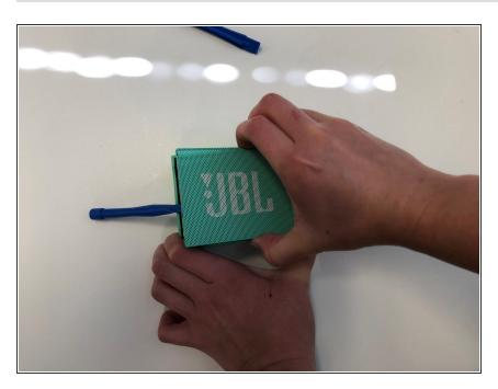
Carefully remove the loose plastic cover from the speaker.
