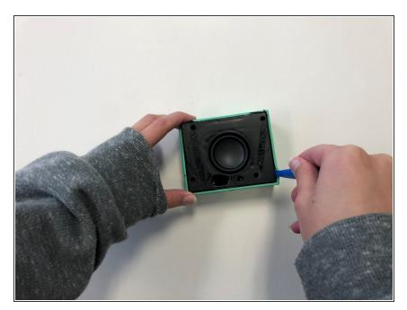
After removing the screws, use the plastic opening tool to carefully pry around the edges of the black cover to loosen and lift the cover off of the device.
