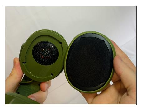
Continue pulling it away from the edges of the plastic covering until the cushion is fully removed.
