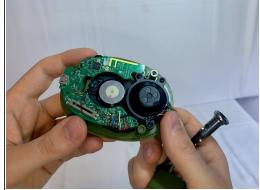
Remove four 4 mm Phillips #1 screws that connect the motherboard with the plastic frame.
