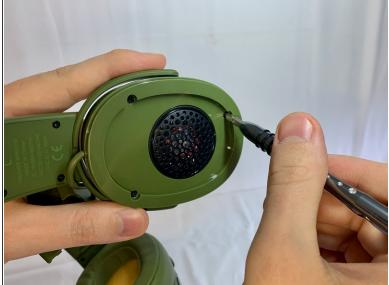
Remove three 12 mm Phillips #1 screws located underneath the left ear cushion.
