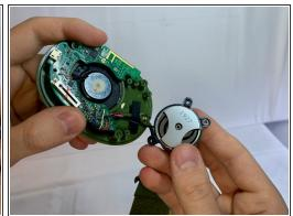
Remove three 4 mm Phillips #1 screws that connect the bass speaker to the plastic frame.
