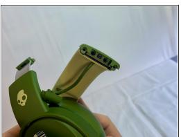
• Remove two 5 mm Phillips #1 screws on the underside of the headband.
