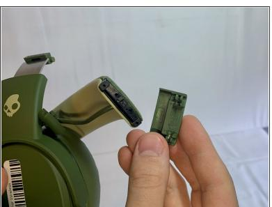
Remove the top plastic part of the hinge.
