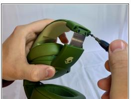
Remove two 14 mm Torx T6 screws on the underside of the headband.
