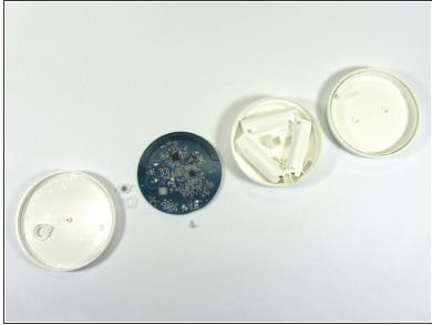
Teardown Exploded Views of the ring Glass Break Sensor
