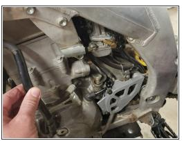
Using needle-nose pliers, loosen the clamp and slide it forward on the fuel line. Then remove the fuel line.
