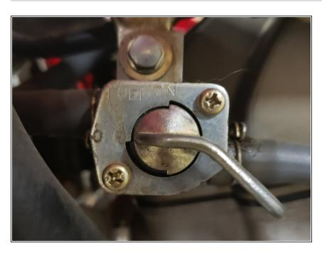
Move the fuel lever from the on position to the off.
