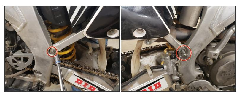
Remove the 10mm lower sub-frame bolts on each side of the motorcycle.
