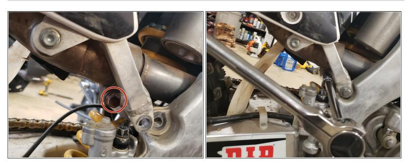
Loosen the 12mm bolt to separate the exhaust muffler from the exhaust header.
