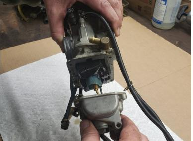
• Loosen and remove the 5 screws at the bottom of the carburetor, with the Phillips head screwdriver, to detach the bowl. Then remove the bowl.
