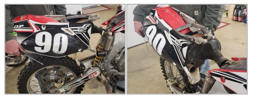
Remove the sub-frame assembly from the rest of the motorcycle.
