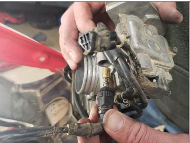
Un-thread the 13mm plastic hot start cable from the carburetor.
