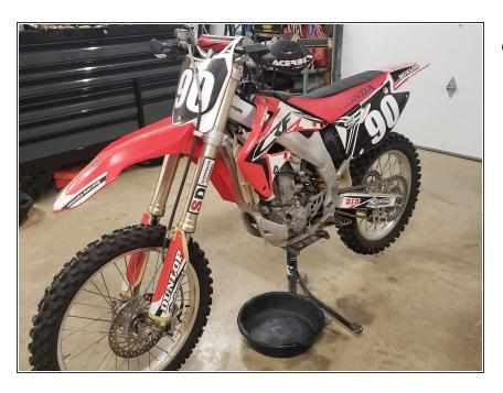
Place a drain pan under the motorcycle to catch any excess fuel.
