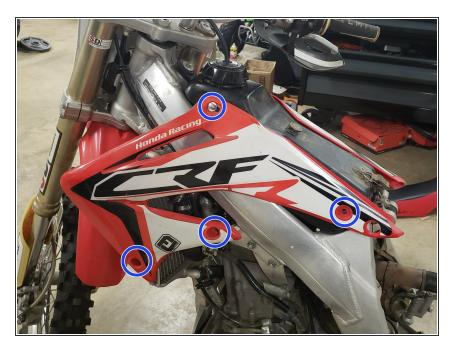
Remove the side shrouds from the motorcycle by loosening the four 8mm screws. Complete this step for both sides of the bike.
