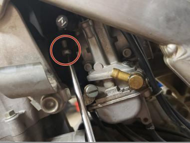
Loosen the clamp on the front of the carburetor with the Phillips head screwdriver.
