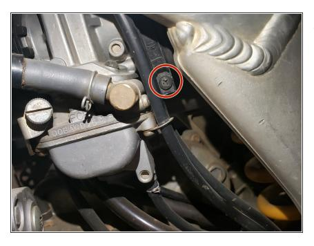
Loosen the screw with a phillips head screwdriver so the clamp can move freely.
