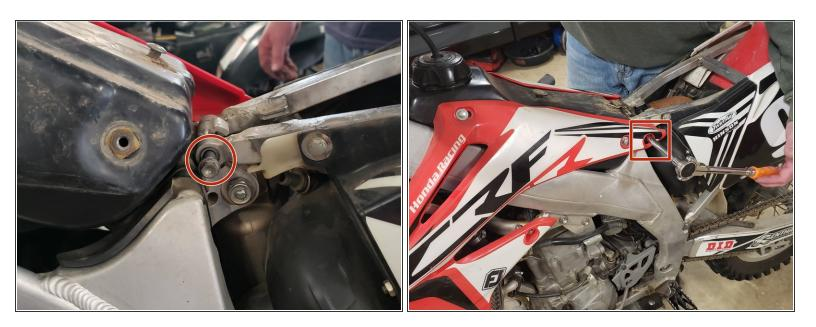
Remove the 10mm upper sub-frame bolt from the motorcycle.
