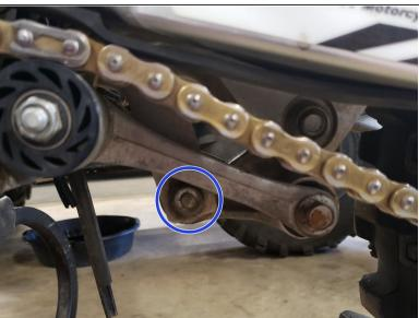
Remove the top and bottom shock bolts with 17mm socket.
