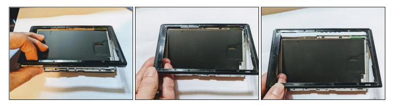
• Lift the front edge of the frame then slide the frame up toward the top of the display to remove it.
